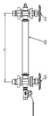
Model 34041 High Pressure Boiler Gauge Fixture Set With Ball Check 250WSP @ 406° F ASME Compliant per B31.1 and Section One, PG 60 Appendix A18 of ASME Boiler Code CRN OCO7137.2C
