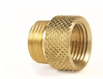
200 lbs. WOG Available in 1/2" NPT Male X 1/2" NPT Female and 3/4" NPT Male X 3/4" Female NPT in Assorted Lengths Brass (ASTM B16)
